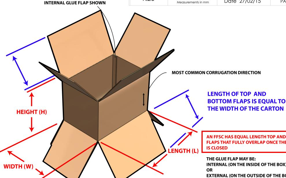
AN FFSC HAS EQUAL LENGTH TOP AND BOTTOM FLAPS THAT FULLY OVERLAP ONCE THE CARTON
